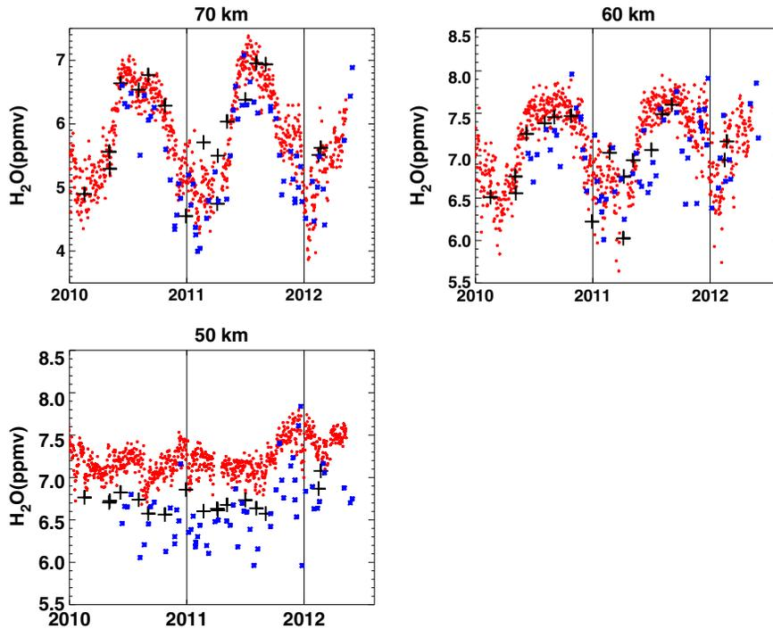
**Figure 4.** WVMS (blue) and coincident MLS (red) and ACE (black) measurements for Table Mountain. Satellite measurements have been convolved with the averaging kernels from the WVMS retrievals.
