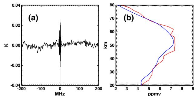
**Figure 3.** Measurements from Table Mountain, 11–16 December 2010. (a) Residual from WVMS measurements and (b) water vapor mixing ratio profiles from WVMS (blue) and MLS (red). The baseline sine wave that was calculated from the fit to the 1–7 June 2011 WVMS measurements (Figure 2) has been added to this WVMS retrieval and successfully remove the largest instrumental baseline component.
