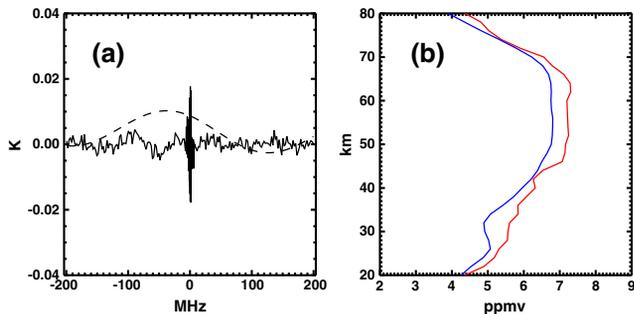
**Figure 2.** Measurements from Table Mountain, 1–7 June 2011 (same dates as Figure 1). (a) Residual from WVMS measurements and (b) water vapor mixing ratio profiles from WVMS (blue) and MLS (red). The WVMS retrieval shown here allows for the fitting of a single sine-wave baseline (indicated by dashed line).
