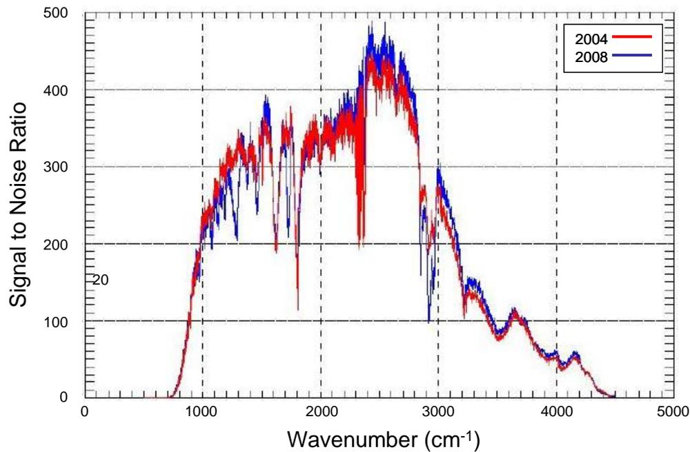
Figure 5: On-orbit SNR comparison of 2004 (blue) and 2008 (red). Each curve was built with exoatmospheric measurements during five occultations at beta angle near  $0^\circ$
