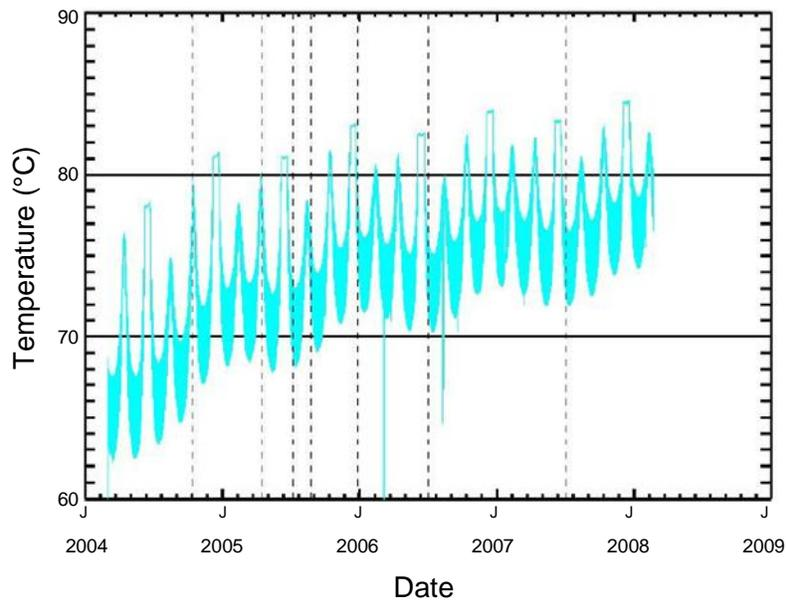
Figure 10: Evolution of the temperature of the sun-tracker mirror with time
