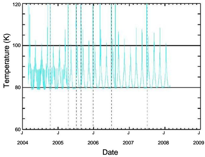
Figure 12: Evolution of the cold stage temperature with time
