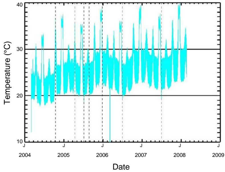
Figure 11: Evolution of the temperature of the aperture stop with time
