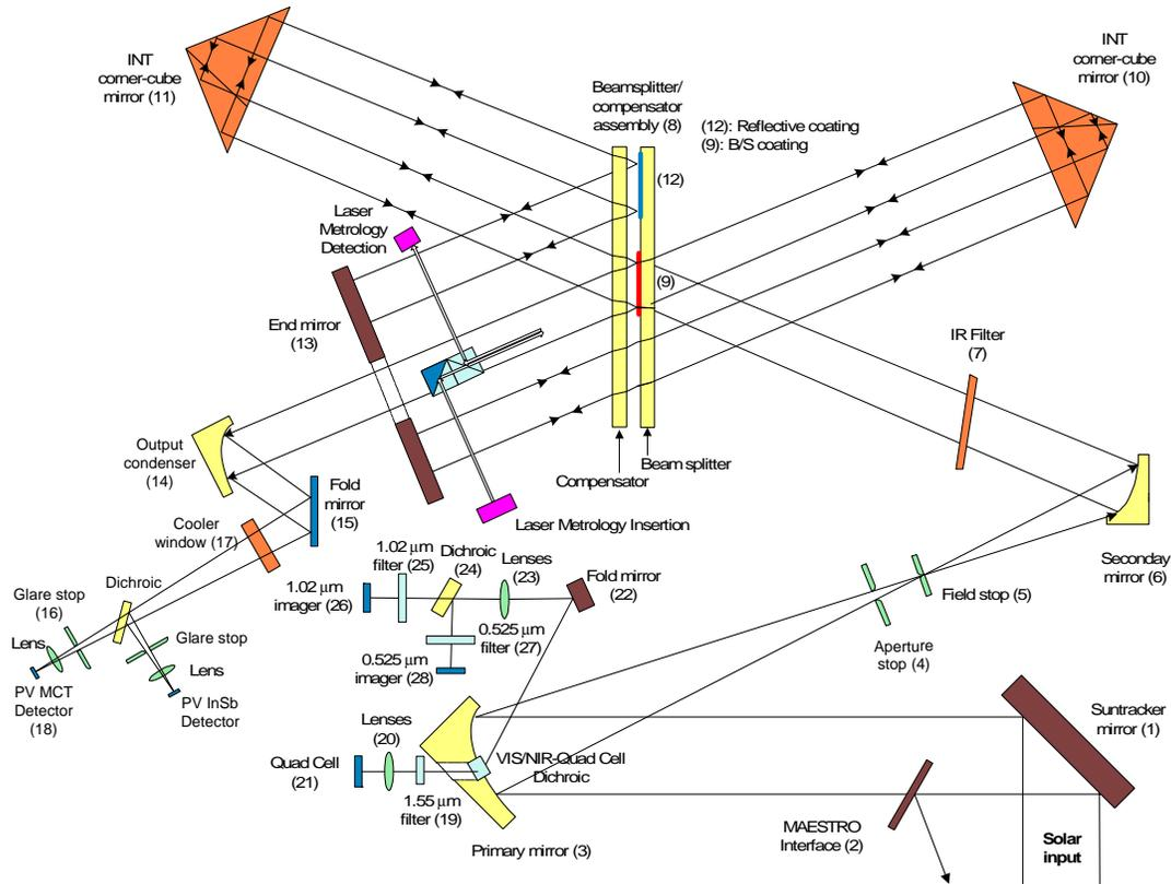
Figure 1: ACE-FTS instrument optical layout
