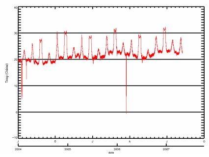
Figure 9: On-orbit FTS temperature (interferometer beamspliter) 2004-2007
