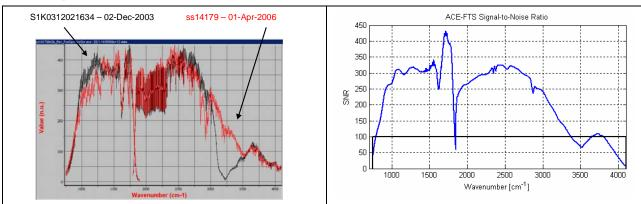
Figure 3: Validation of SNR model: on-orbit SNR (left) and modeled SNR for scene at 5800 K (right)
