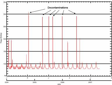
Figure 6: Evolution of the cold stage temperature with time
