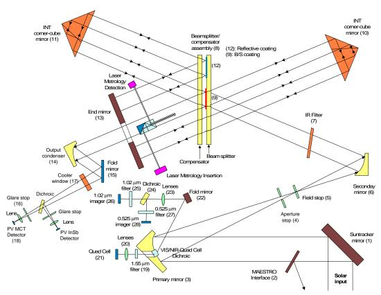
Figure 1: ACE-FTS instrument optical layout
