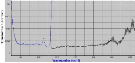
Figure 7: On-orbit FTS transmittance accuracy
