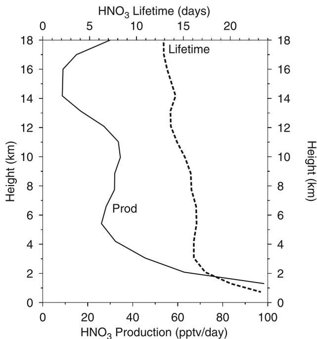
**Figure 15.** Rate of production of nitric acid (solid curve) and its lifetime against photochemical loss (dashed curve). These were used to calculate the mean nitric acid profiles of the CONRAD (Emanuel) and TCM (Folkens and Martin) models. Below 14 km, the profiles were generated using the GEOS-Chem off-line chemical transport model using GEOS-4 meteorology. Above 14 km, they were calculated from ASHÖE/MAESA and STRAT measurements using a procedure discussed in the text.
