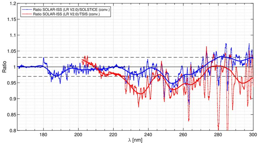
**Figure 7** Ratio to SOLAR-ISS (V2.0) for *SORCE/SOLSTICE* (blue curve) and *TSIS* (red curve). These ratios are based on comparison between existing extraterrestrial solar spectra based on observations (*SOLAR-ISS* (April 2008), *SORCE/SOLSTICE* (April 2008), *TSIS* (March 2018 to March 2019)). The black dashed lines show the uncertainties at  $\pm 3\%$ .
