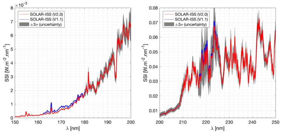
**Figure 3** *Left:* Solar spectral irradiance of the two versions of the SOLAR-ISS spectrum in the 165–200 nm spectral region. *Right:* Comparison between the two versions of the SOLAR-ISS spectrum in the 200–250 nm spectral region.
