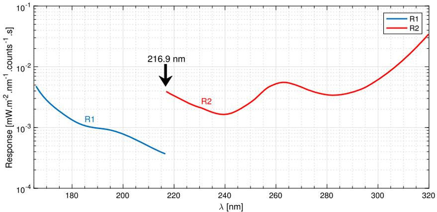
**Figure 4** The *blue curve* corresponds to the SOLAR/SOLSPEC absolute response (R1) in the 165–216.6 nm range. The *red curve* corresponds to the SOLAR/SOLSPEC absolute response (R2) in the 216.9–320 nm range.
