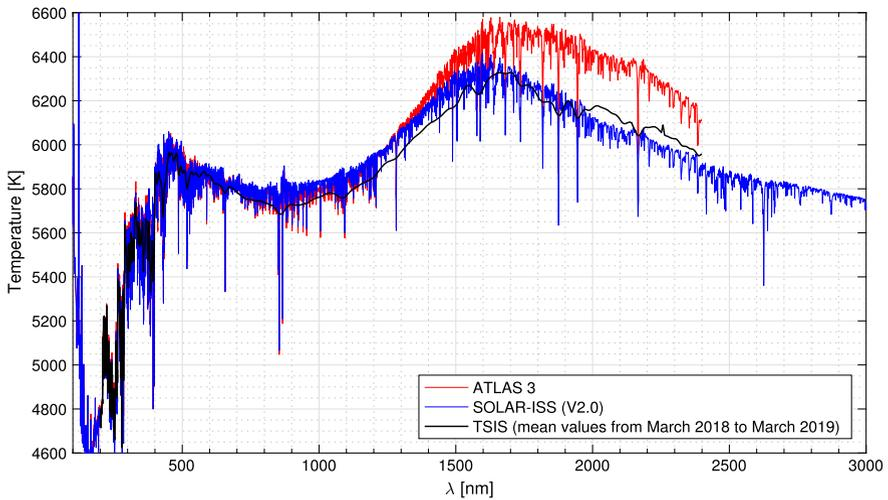
**Figure 8** Brightness temperature of the Sun obtained from the ATLAS 3 (period: November 1994) solar spectrum data plot (red curve), SOLAR-ISS (period: April 2008) spectrum data (blue curve) and TSIS (period: March 2018 to March 2019) spectrum data (black curve).
