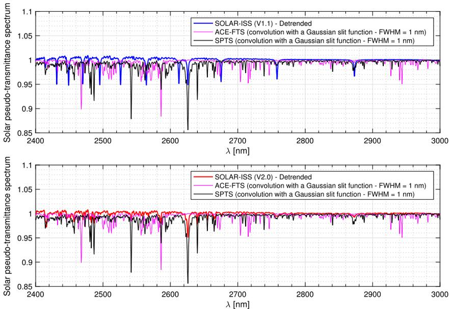
**Figure 5** *Top:* Detrended SOLAR-ISS spectrum (V1.1) with a low-order polynomial fit and solar pseudo-transmittances (ACE-FTS and SPTS) in the 2400–3000 nm spectral region. *Bottom:* Detrended SOLAR-ISS spectrum (V2.0) with a low-order polynomial fit and solar pseudo-transmittances (ACE-FTS and SPTS) in the 2400–3000 nm spectral region.
