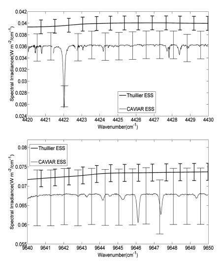
**Figure 7.** The CAVIAR ESS (thin line) and Thuillier ESS (thick line) with their (k=2, 95% confidence level) uncertainties from 4420–4430 cm<sup>-1</sup> (about 2.26 µm) (top) and 9640–9650 cm<sup>-1</sup> (about 1.04 µm) (bottom). The CAVIAR ESS has been derived from observations of 18 September 2008.
