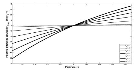
**Figure 2.** The percentage difference between  $F_{0new}$  and  $F_0$  for different constant optical depths,  $\tau_0$  and parameter, k using airmass m and k values typical of the observations of 22 August 2008 and assuming up to a 20% change in the water vapor amount. The relative difference is  $(F_{0new} - F_0)/F_{0new}$ . See text for details.
