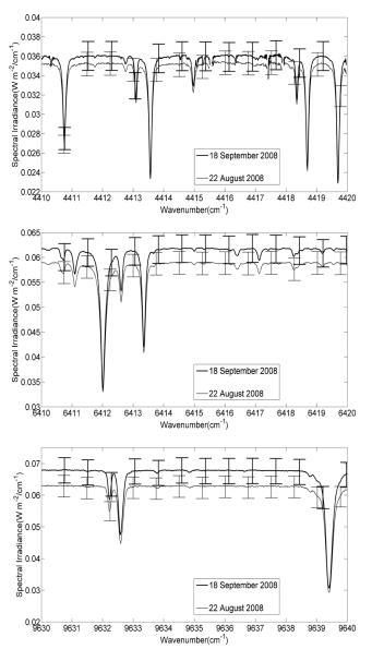
**Figure 8.** The CAVIAR ESS derived from observations of 18 September 2008 (thick line) and 22 August 2008 (thin line) with their respective (k=1, 67% confidence level) uncertainties in three spectral regions: (top) 4410–4420 cm<sup>-1</sup> (about 2.27 µm), (middle) 6410–6420 cm<sup>-1</sup> (about 1.56 µm), and (bottom) 9630–9640 cm<sup>-1</sup> (about 1.04 µm).
