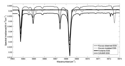
**Figure 6.** A comparison of the CAVIAR ESS (thick line) with the Kurucz-observed ESS (thin line), the Fontenla ESS (very thick line), and the Kurucz-modeled ESS (very thin line) in the spectral region  $5963-5973 \text{ cm}^{-1}$  (1.67–1.68 µm). The CAVIAR ESS has been derived using observations of 18 September 2008.
