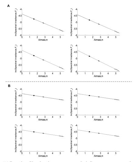
**Figure 4.** (A) Examples of Langley plots at some atmospheric line centers at wavenumbers (in  $\text{cm}^{-1}$ ) 2524.6 (top left), 2525.7 (top right), 2526.0 (bottom left), and 2526.8 (bottom right). (B) Examples of Langley plots at some atmospheric microwindows, at wavenumbers (in  $\text{cm}^{-1}$ ) 2526.4 (top left), 2527.3 (top right), 2529.4 (bottom left), and 2531.5 (bottom right). Both sets of Langley plots have been obtained from 18 September 2008 observations.
