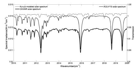
**Figure 1.** CAVIAR extraterrestrial solar spectrum (thick line and left axis) from Camborne observations of 18 September 2008 in the spectral region  $2510-2520 \text{ cm}^{-1}$  (3.97–3.98 µm) compared with the Kurucz-modeled (very thin line and left axis) and ACE-FTS (thin line and right axis) extraterrestrial solar spectra.
