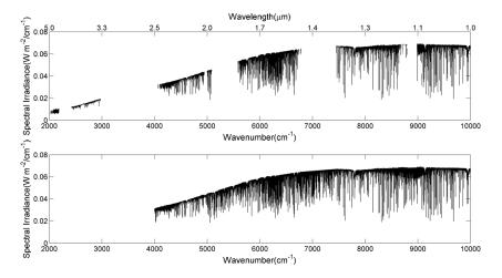
**Figure 9.** (top) CAVIAR ESS at one astronomical unit (1 AU) from  $2000-10,000 \text{ cm}^{-1}$  (1–5 µm). (bottom) The merged CAVIAR ESS from  $4000-10,000 \text{ cm}^{-1}$  (1–2.5 µm). This ESS is a merger of the CAVIAR ESS derived using observations of 18 September 2008 with the ACE-FTS ESS, Kurucz-observed ESS, and Kurucz-modeled ESS.
