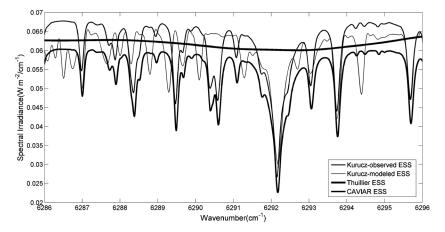
**Figure 5.** A comparison of the CAVIAR ESS (thick line) with the Kurucz-observed ESS (thin line), Thuillier ESS (very thick line), and the Kurucz-modeled ESS (very thin line) in the spectral region  $6286-6296 \text{ cm}^{-1}$  (1.58–1.59 µm). The CAVIAR ESS has been derived from observations of 18 September 2008.
