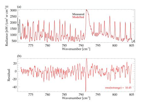
Figure 5. Impact of the  $CO_2$  Q-branch at 11.5 km altitude taking line mixing it into account: (a) spectra; (b) residuals. Black: measured spectrum, hardly discernible because overplotted by modelled spectra. Note the different scale of the residual axis compared to Fig. 4.
