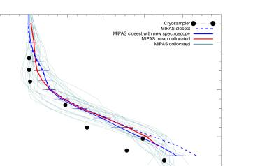
Figure 16. Comparison of MIPAS Envisat and cryosampler  $CCl_4$ . The cryosampler measurement was taken on 1 April 2011. The continuous and dashed blue lines are the respective closest MIPAS Envisat profiles calculated using the new and the old spectroscopic data set.
