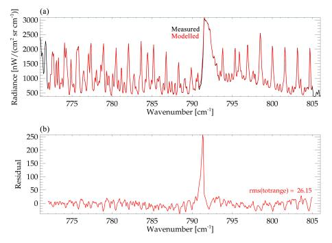
Figure 4. Impact of the  $CO_2$  Q-branch at 11.5 km altitude without considering line mixing: (a) spectra; (b) residuals. Black: measured spectrum, hardly discernible because overplotted by modelled spectra.
