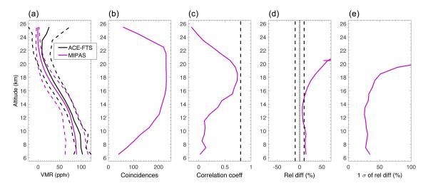
**Figure 13.** Comparison of MIPAS Envisat and version 3.5 ACE-FTS  $CCl_4$ . (a) Mean profiles of all coincident profiles (black: ACE-FTS; magenta: MIPAS). Dashed lines show the standard deviations of the mean profiles. (b) Number of coincident points per altitude. (c) Correlation coefficient of the mean profiles. (d) Relative differences of the mean profiles. (e) One standard deviation of the relative differences of the mean profiles.
